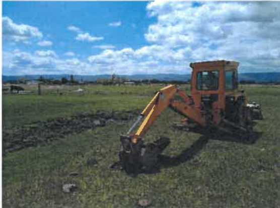
Excavator-assisted soil sample.
